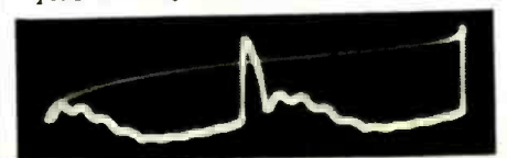
Fig. 14. Waveform at plate of horizontal output tube. Condenser shorted and series resistor across half of horizontal yoke winding subsequently was burned.
