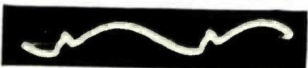
Fig. 12. Waveform at plate of horizontal output tube. This pattern is obtained when there is a shorted condenser between "B+" and boosted "B+" circuit.
